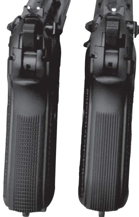
More subtle differences between the M9A1 on left and M9 on right include a checkered rather than a ribbed backstrap and twin white dot rear sight inserts instead of a single white half moon. (Author’s photo)
