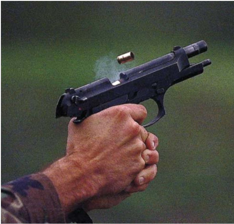
This photo of the M9 being fired by a member of the US Air Force offers a good view of the slide cycling and the spent cartridge case being ejected. (USAF)
