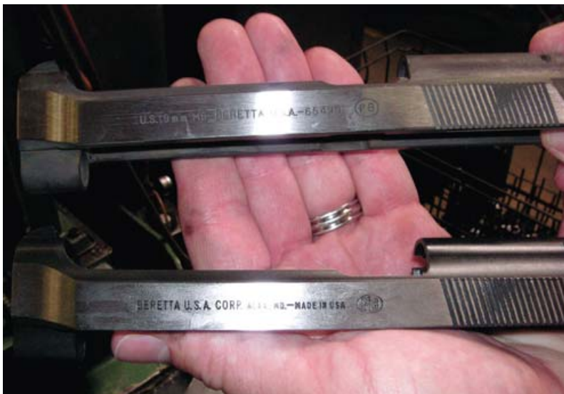
Beretta USA machines Model 92 and M9 slides on the same machinery; note that it marks them differently. (Author's photo)
