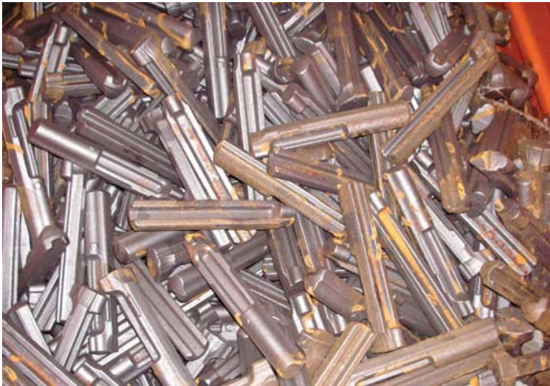
Castings for M9 slides awaiting machining at Beretta USA. The fracturing of the SEALs' Italian-made M9 slides was the first operational failure suffered by the new 9mm. By 1988, however, slides were being manufactured at Beretta USA, and no further problems were encountered. (Author's photo)
