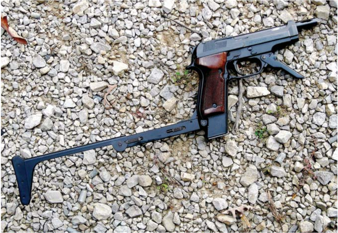
The Beretta 93R, which allows three-round burst fire; note the shoulder stock and folding vertical foregrip. (Author's photo)
