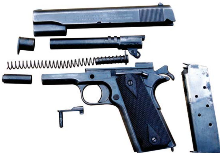
This Colt 1911 pistol has been disassembled – “field-stripped” – for cleaning.
