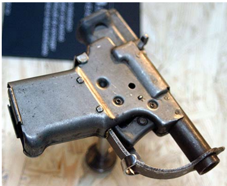
The OSS's .45 ACP Liberator pistol, intended for resistance fighters. The OSS and its British equivalent, the SOE, also found the .45 ACP to be an ideal cartridge for clandestine use with silenced weapons, for it was subsonic and did not create the resonant “crack” in flight that gave away the firing of supersonic cartridges. The OSS and SOE were both supplied with silenced weapons that chambered the .45 round, predominantly the Thompson and M3 “Grease Gun” submachine guns. Even when fired on full-automatic, these guns made no more noise than an air rifle and would have been undetectable in a busy environment. (Rama)
