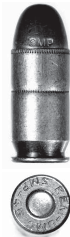
W. E. Fairbairn arranged for specially marked .45 ACP ammunition to be issued to the SMP so it could be determined from used bullets and cases whether shots had been fired by the police. (Woodin Labs)
