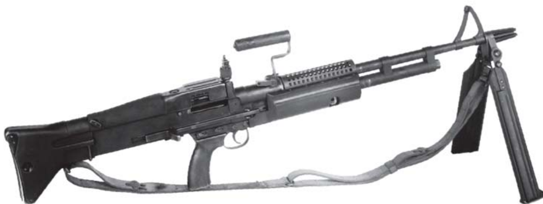
The T52E3 fitted with the light barrel. The front sling swivel idea was quickly dropped from the design since it prevents the barrel from being completely released from the weapon. The barrel-release lever is on the top of the front of the receiver, visible at the base of the carrying handle. (US Government)
