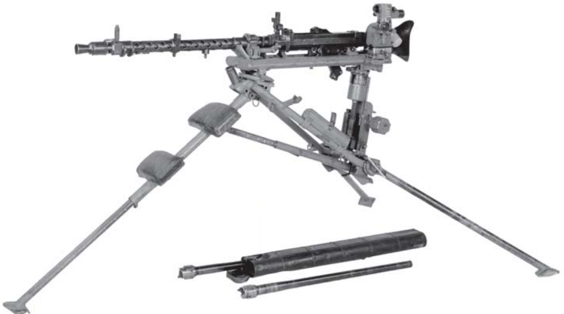
The MG 34 on the complex Lafette 34 tripod. The tripod is fitted with an optical periscope sight, visible to the left of the gun just in front of the rear of the butt stock. The barrel carrier shown underneath the tripod holds two barrels. (US Army)
