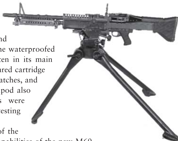
A left-side view of the M60 light machine gun mounted on an M91 tripod. The legs of the tripod can be adjusted to raise or lower the height of the weapon. The tall tripod arrangement allows the weapon to be used for accurate indirect fire, firing at long range where the target cannot be seen by the gunner. This is possible in part because of the precise controls in the mount cradle at the top of the tripod which set the angle and direction of the weapon. This very early specimen of the M60 has neither the magazine bracket on the left side of the receiver, nor the bandoleer hanger under the feed tray, to hold an ammunition belt. For firing, this weapon would be fed from a long belt held in an ammunition can sitting on the ground and guided by the assistant gunner. (US Government)
