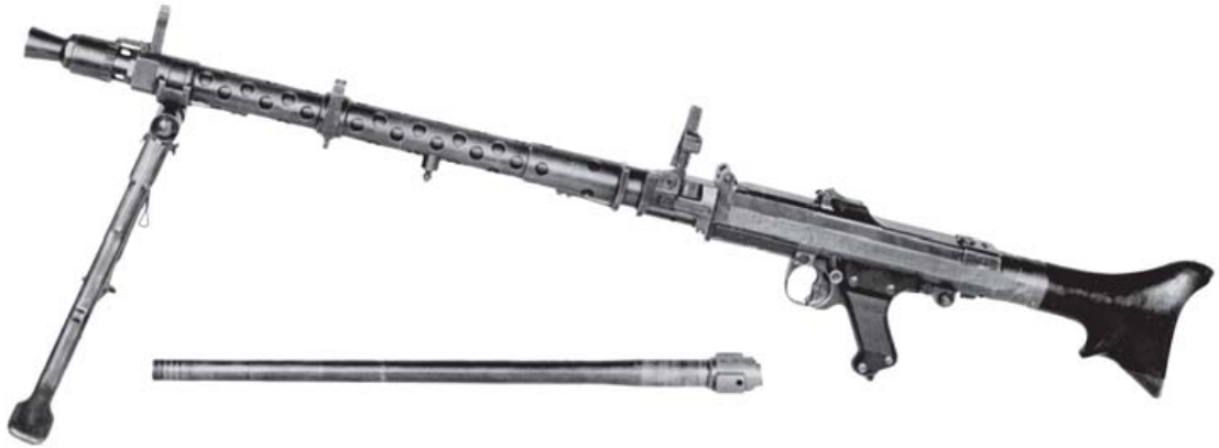
The MG 34 light machine gun. A carefully crafted weapon, the MG 34 is primarily made of finely machined parts. The spare barrel is shown underneath the weapon. (US Army)
