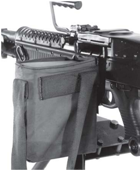
The M4 bandoleer attached to the hanger on the side of an M60 machine gun in place to feed ammunition into the weapon. The M60 is mounted on an M122 tripod; one of the controls to the traverse and elevation mechanism is the round knob visible under and behind the pistol grip of the weapon. (US Government)
