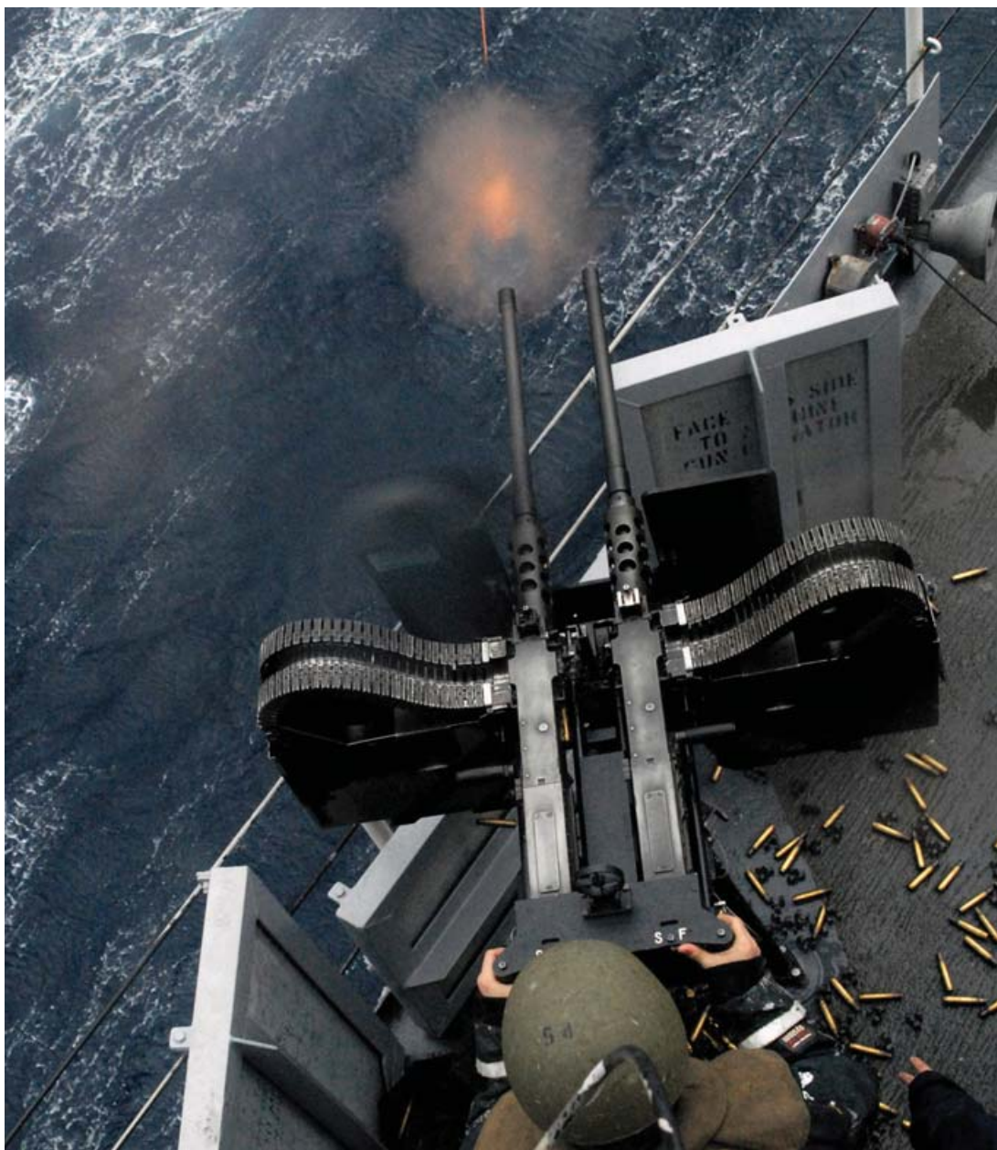
A gunner aboard the amphibious transport dock ship USS Juneau fires a twin .50-cal HB M2 machine gun during a live fire training exercise. This mount requires that the right gun be reconfigured for right-hand feed. (US Navy/Michael D. Kennedy)
