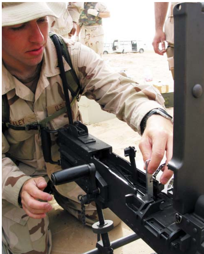
A gunner's mate tests the barrel alignment of an HB M2 .50-cal machine gun with the "GO-NO GO" headspacing gauge during a joint live-fire exercise at Camp Patriot, Kuwait. The two timing gauges are attached to the other end of the chain. (US Navy/ Joseph Krypel)
