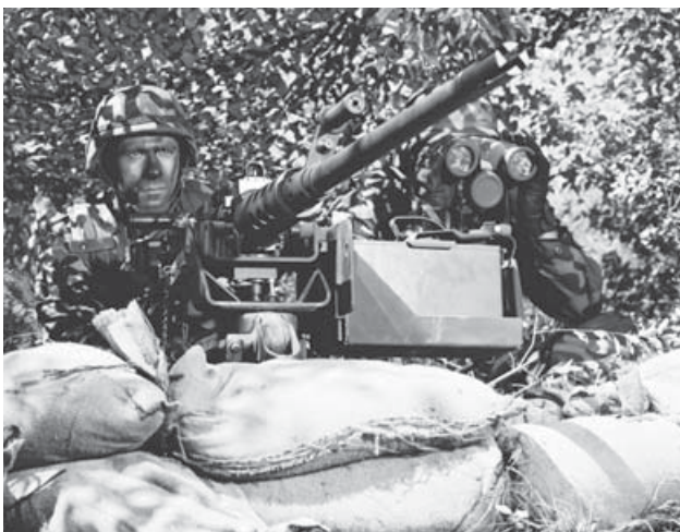
A .50-cal M2E2 machine gun includes the Quick Change Barrel Kit Program with redesigned barrel changing handle, manual trigger block safety, night-vision sight-friendly flash suppressor, and set headspace and timing. (Courtesy General Dynamics)
