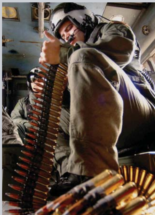
ABOVE An Aviation Warfare Systems Operator inspects .50-caliber machine gun rounds in preparation for a live fire exercise. Rounds are inspected for proper seating in the link, cleanliness, damage, and corrosion. This is a standard mix of one M20 API-T and four M8 API. (US Navy/Jayme Pastoric)
