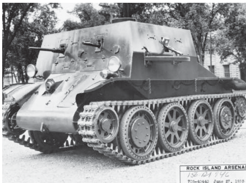
A 1935 experimental T4 combat car mounted four .30-cal M1919A4 machine guns plus a .50-cal M2 machine gun in the right bow. The gun is fitted with the 36in-long finned barrel. (Cody Images)
