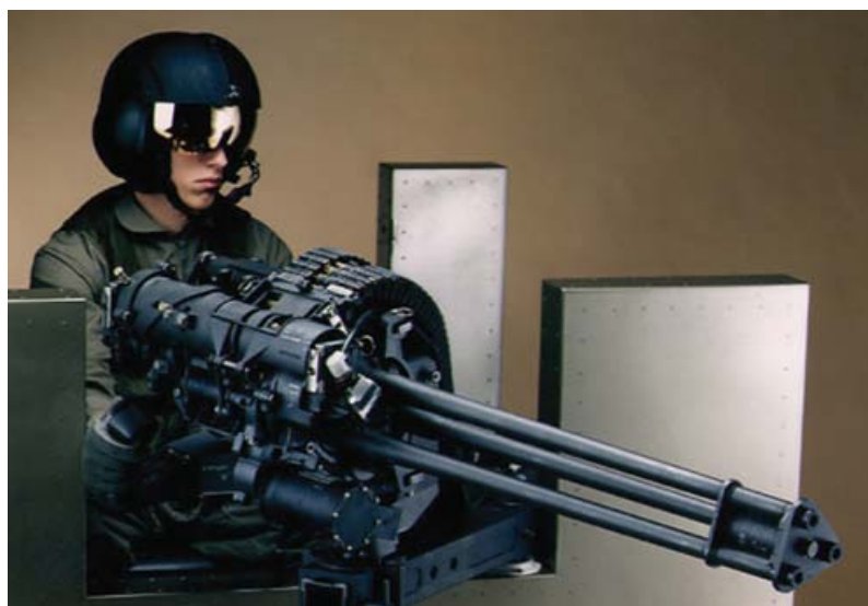
The General Electric .50-cal GAU-19/A. This three-barrel rotary machine gun is far too heavy to be an effective replacement for the M2. One of the hazards of these high-speed rotary guns is that tiny fragments of the cases are ejected during firing. (Courtesy General Dynamics)
