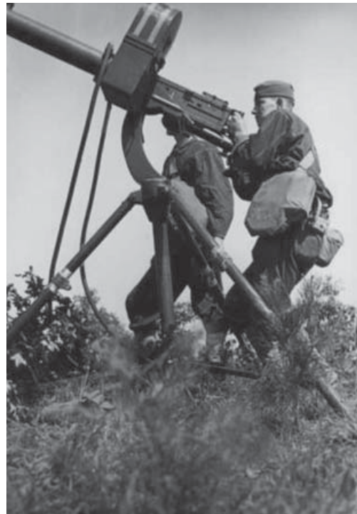
The first standardized .50-cal Browning was the M1921 water-cooled anti-aircraft machine gun with a 36in barrel, here on an M1 AA tripod. It can be seen how the legs hampered the gunner when tracking a high-speed aircraft. It is fitted with a 200-round M2 "tombstone" ammunition case. (US Army)
