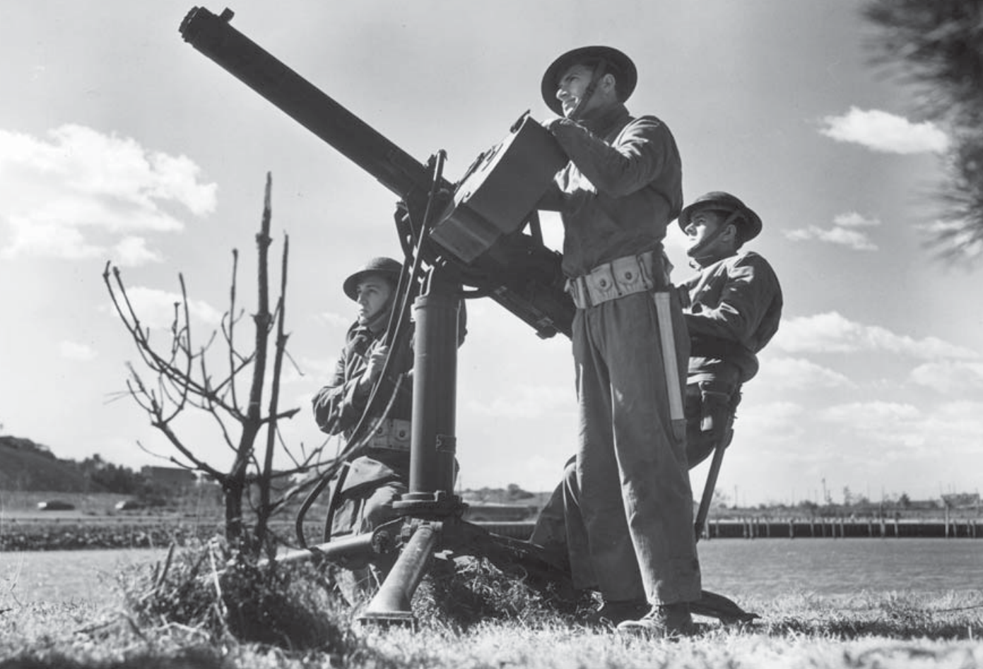
Three soldiers of the 62nd Coast Artillery Regiment (Antiaircraft) manning a .50-cal M2 water-cooled gun mounted on an M2 antiaircraft mount and fed by a 200-round M2 "tombstone" ammunition chest. A full chest weighed 87lb. (Hulton Archive/Getty Images)
