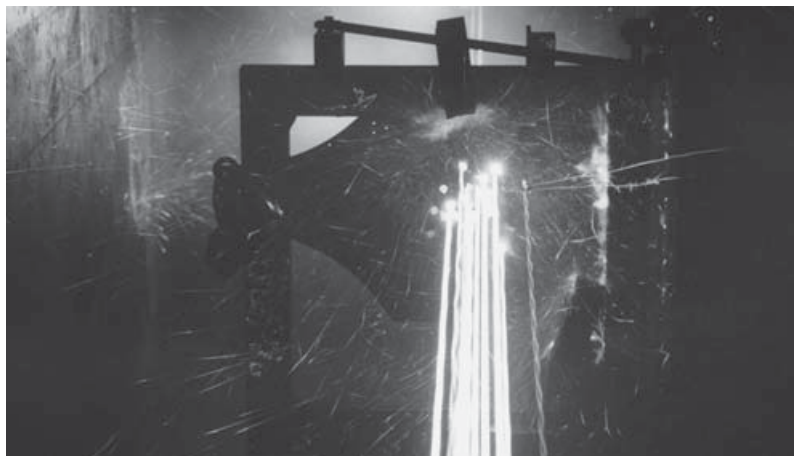
Slicing through metal – .50-cal tracer bullets are fired through aircraft armor plate during testing. (Photo by Dmitri Kessel/Time Life Pictures/Getty Images)
