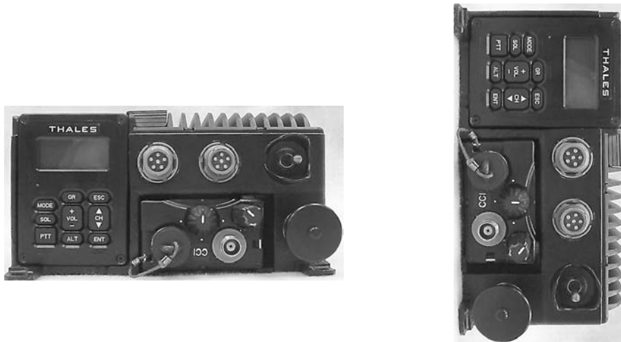
Figure 6-1 VA Horizontal Mounting Configurations
