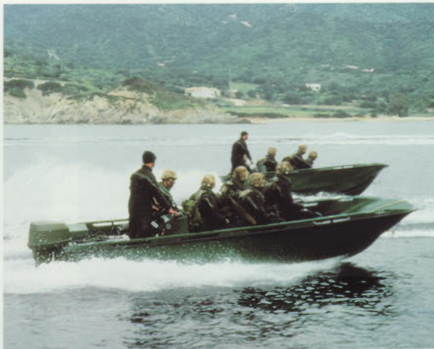
The fiberglass fast assault boats can travel at more than thirty-knots with up to eight fully-equipped troops. Light, fast and maneuverable, these crafts are ideal for commando operations.
