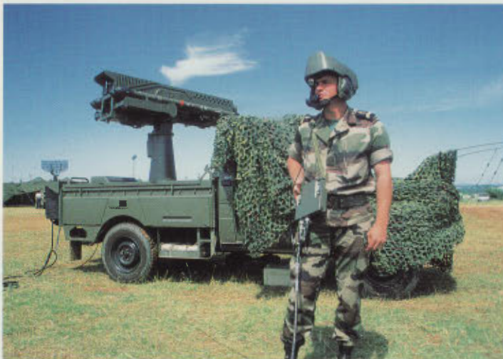
"EOLE 98" introduced, for the first time, the ASPIC light antiaircraft system—four Mistral antiaircraft missiles mounted on a Peugeot P-4 vehicle. The battery featured here belongs to the air defense detachment of the sprawling Istres Air Force Base. Note the Ares helmet worn by the commander of the vehicle.
