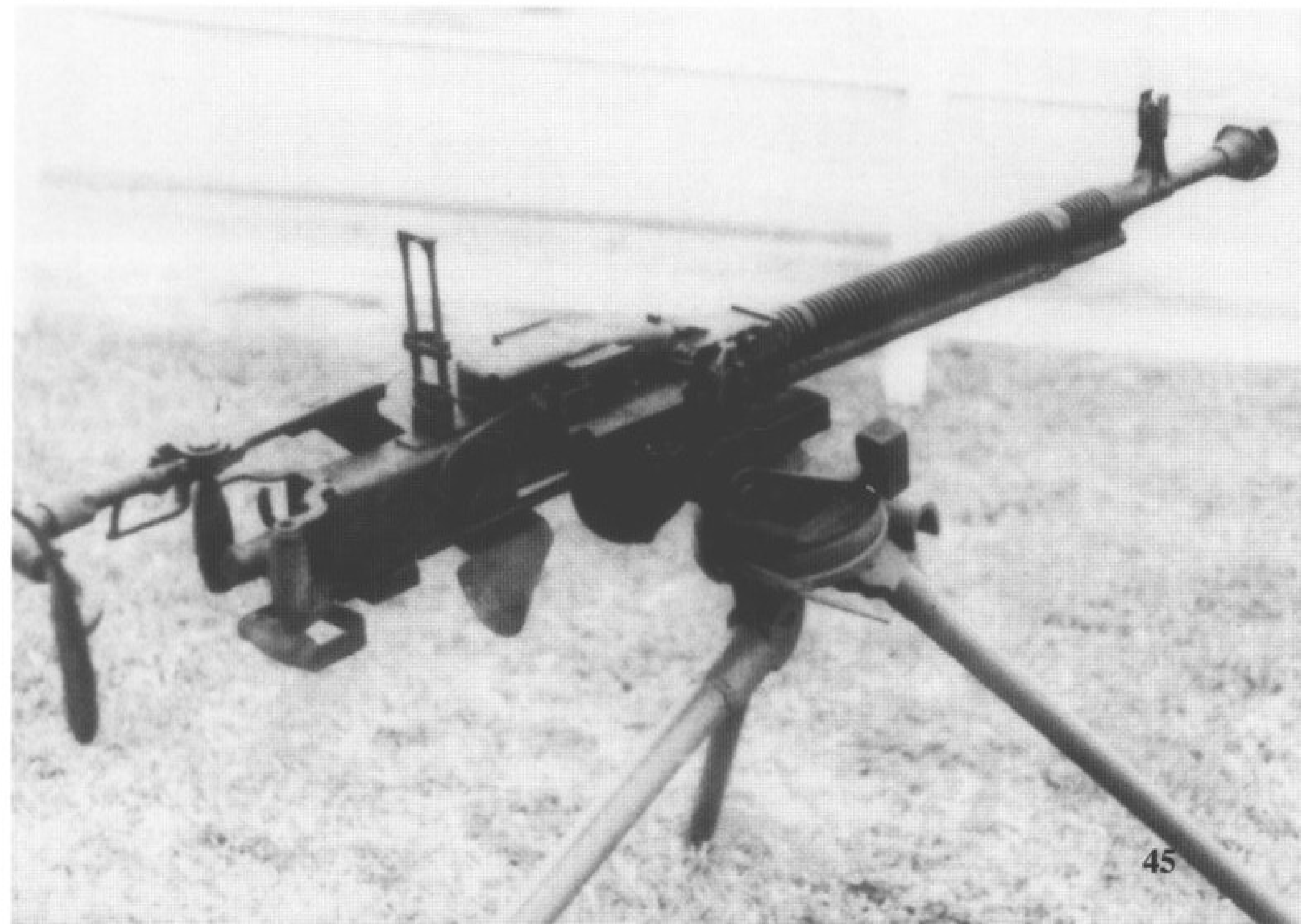
Captured equipment was always welcomed by the intelligence groups. This is a Chinese made 12.7mm machine gun used as an anti-aircraft weapon. It was captured at an enemy base camp. This type of machine gun was particularly effective against low flying helicopters. (Joe Troxell)
