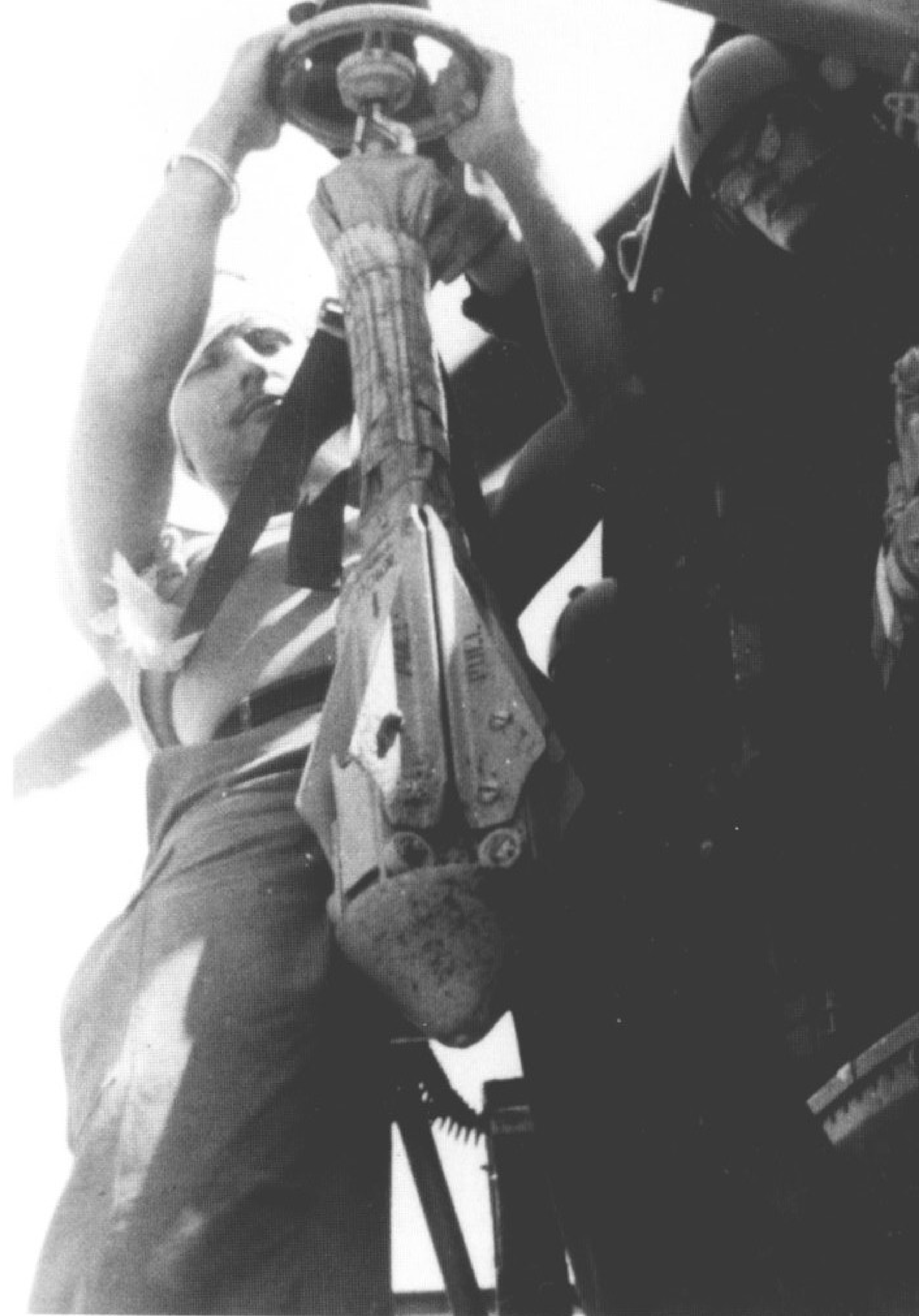
A wounded man is hoisted on board the UH-1D Dustoff Medevac helicopter via the jungle penetrator. Quick medical evacuation of a wounded man could make the difference in life or death. The jungle penetrator was the best way to pluck a wounded man from the thick jungle terrain. (U. S. Army)
