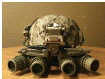
A ballistic helmet outfitted with the latest generation of night-vision goggles, helmet-mounted flashlight, and IR strobe. The four tubes on these NVGs allow better peripheral vision than the standard two-tube goggles. The IR strobe is vital when dealing with helicopters and other aerial assets.
