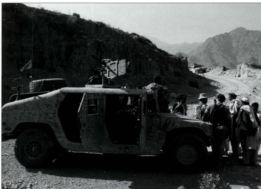
A mounted SF patrol halts to talk with locals. They are travelling in an up-armored HMMWV mounting a Mk 19 automatic grenade-launcher (AGL), and finished in field-expedient camouflage of closely applied small brown 'curls' on khaki. (Courtesy 'JZW')
