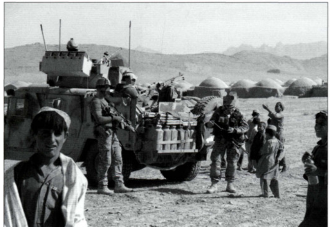
Poland: GROM operators providing security for visiting VIPs; although it is obscured here, the unit wear the unusual and recently adopted Crye Multicam pattern battledress uniform, previously only extensively used by the US Army CAG. The up-armoured GMV – a Humvee modified to SF standards – mounts a .50cal M2 in its armored turret, and a 7.62x54mm PKM for the rear gunner; note also the fuel cans in the rear rack. (Polish Ministry of Defence photo)
