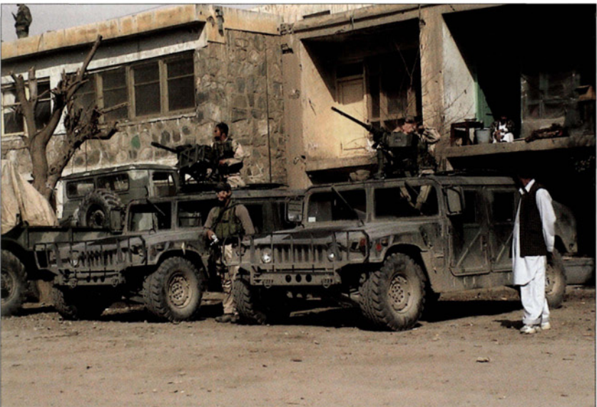
An excellent view of two up-armored HMMWVs, the left one mounting a Mk 19 AGL and the right a .50cal M2. One ODA member explained that the lead vehicle in a column usually had a Mk 19, the rear one – the ‘caboose’ – a .50cal M2, and the others M240s or M249s; extra ammunition and Claymores were also carried in the Humvees. In fact, few SF Humvees are up-armored; SF prefer to rely on speed, arguing that the extra armor weighs the vehicle down to an unacceptable level, though most teams will have an M1114 armored version available for special tasks. (Courtesy ‘JZW’)
