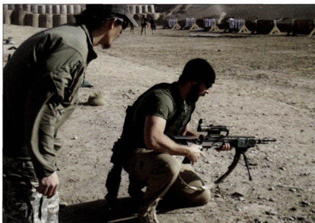
USAF pararescue-jumper of the 306th Rescue Sqn zeroing weapons at Kandahar; he carries a slung M4A1 while he examines a newly issued 7.62x51mm Mk 14 Mod 0 Enhanced Battle Rifle. Built by Troy Industries for the SEALs, the EBR is a shortened development of the trusty old M14, with a collapsible stock and a rail capability for mounting accessories. (USAF photo/Senior Airman Andrea Wright)
