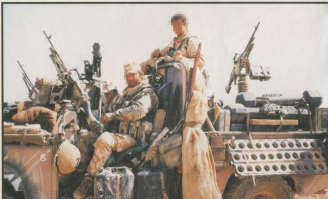
A good shot showing the amount of kit that got draped over the 110s. There are 7.62mm GPMGs front and rear. The cam-nets are rolled up and tied to the roll bar, the sand channels are over the back wheels and above them, looking like dumb-bells, LAW 90 light anti-tank weapons.
