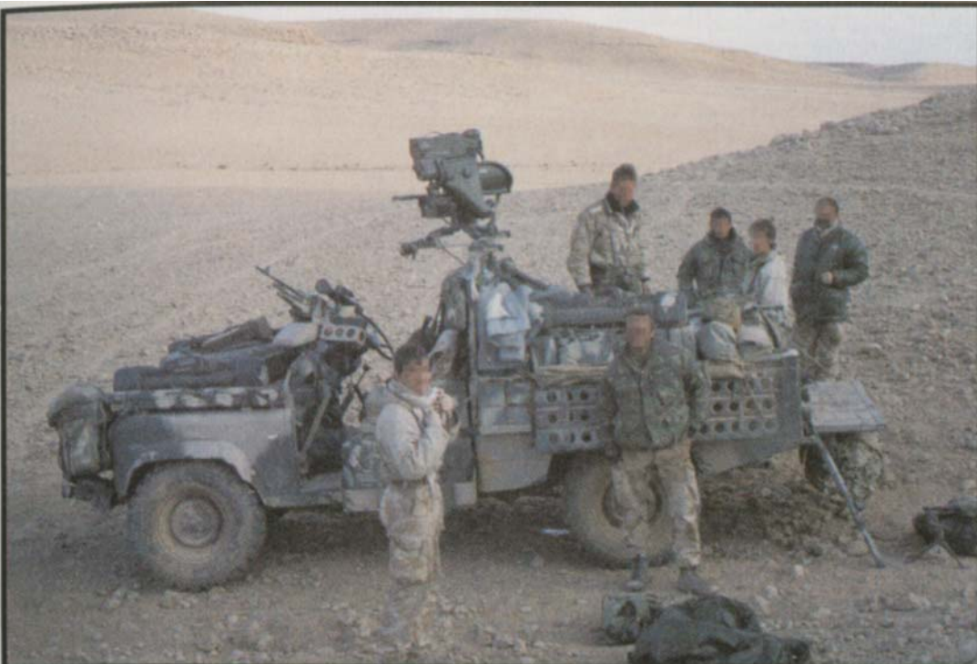
Taff's vehicle. Attached to the roll bar is the Milan missile system, an anti-tank weapon. Fixed to this is the MIRA, a detachable thermal heat image sight. A very good bit of kit.
