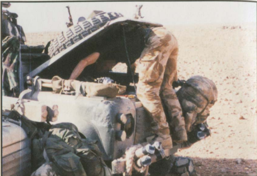
A member of the mobility troop checks a 110 engine. The grenade-launchers on the bumper were for laying down a smokescreen when in contact with the enemy. The plastic desert rat on the bonnet, meanwhile, was just for a laugh.
